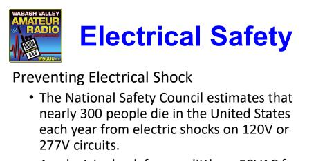
An electric shock from as little as 50VAC for as short a time as 1 second can disrupt the heart's rhythm, causing death in a matter of minutes.
