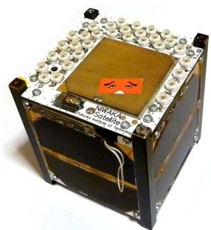
FITSAT-1 was deployed from the ISS on October 4. FITSAT-1 is a small artificial satellite developed at the Fukuoka Institute of Technology in Japan. Nicknamed "NIWAKA", FITSAT-1 is a 10cm cube weighing in at 1.33kg. The main mission of FITSAT-1 will be to demonstrate a 5.8 GHz high-speed transmitter, which can send a jpeg VGA-picture (480x640) within 6 seconds.
