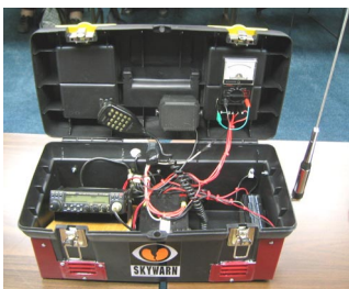
John Van Sandt, N9YRX A self-contained 2M/70cm portable, self-powered rig.
