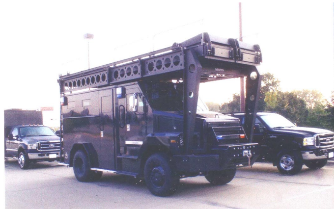
•Illinois State Police armored truck. Entry ladders on roof are hydraulically operated. Probably does not get 38 mpg. More like, 38 gpm, probably.
