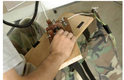
Christian is operating CW using a set of keyer paddles that he designed and built himself.
